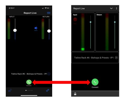
7. Adjust the level of the audio you are sending the studio by using your finger to adjust the "Input" slider. Adjusting the level of the audio the studio is sending you can be completed by adjusting the "Return" slider with your finger.
